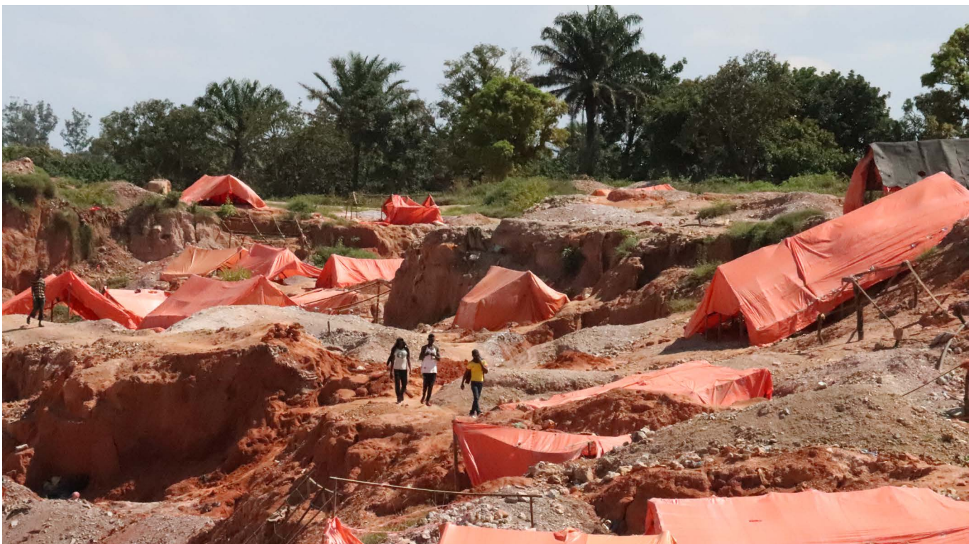
Figure 2 - Each orange tarpaulin hut covers a mining tunnel leading 30-50 meter underground ground. Kasulu Mine, Kolwezi.
