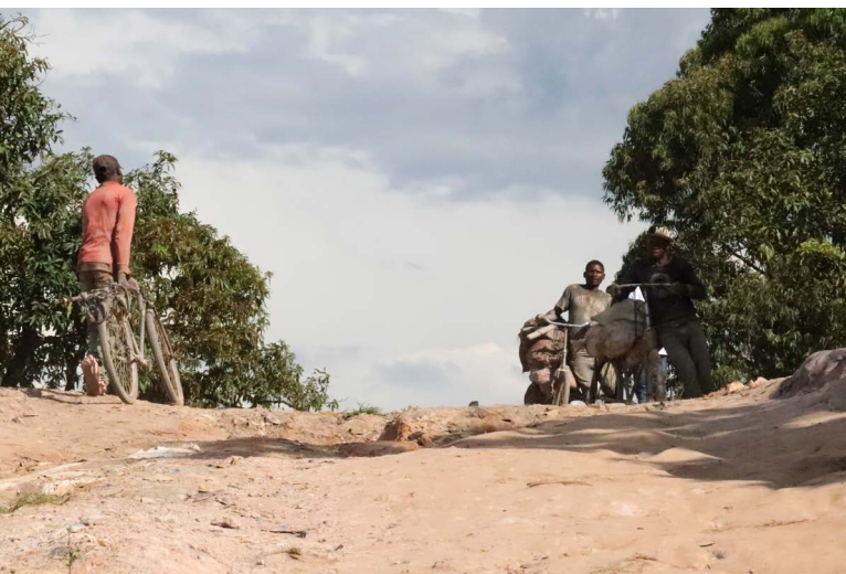
Figure 5 - Often operated by at least two people, bicycles are widely used to transport ore from the tunnels to the warehouses.
